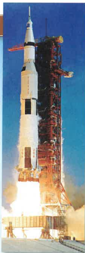
▲ To reach the Moon, NASA developed the giant Saturn V rocket, which lifted a three-person capsule, called Apollo , and a landing craft, called the Lunar Module, into space. Once Apollo and the Lunar Module entered orbit around the Moon, the Lunar Module carried two astronauts from the Apollo capsule down to the Moon's surface.
